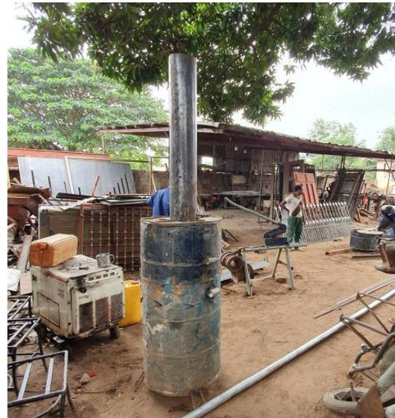
Figure 10: TLUD pyrolyzer at an local workshop ©Bier
